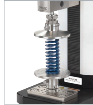
Compression spring testing
